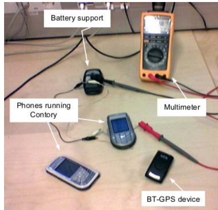
Fig. 3. Power measurements testbed setup
